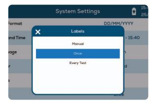
This option sets when and how often the user is prompted to add a label to a test result after a water test is carried out.
