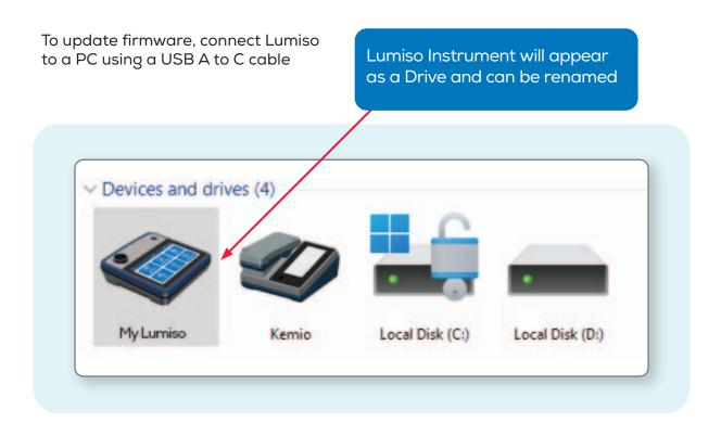
If a new Firmware file has been downloaded or sent electronically, drag and drop that file in to this drive.
