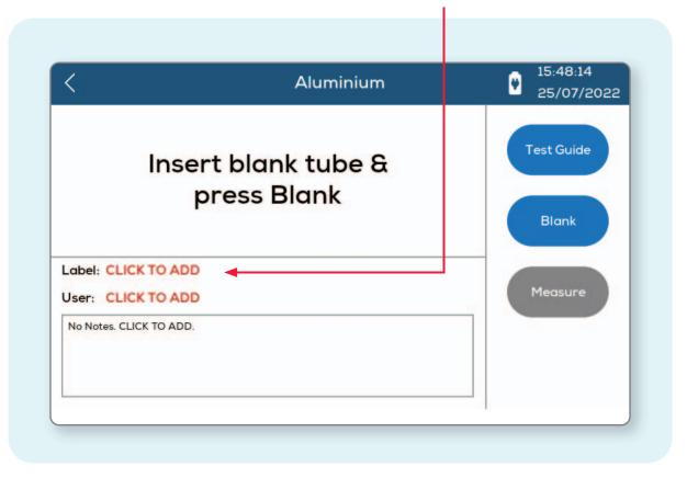
Lumiso can be set to prompt the user to attach a label to each result. (See: Setting Pass and Fail Limits for a Test).
