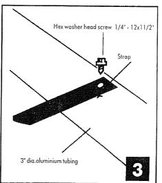
You must drill holes in aluminium tubing to fix straps which are already attached to sollar cover.
