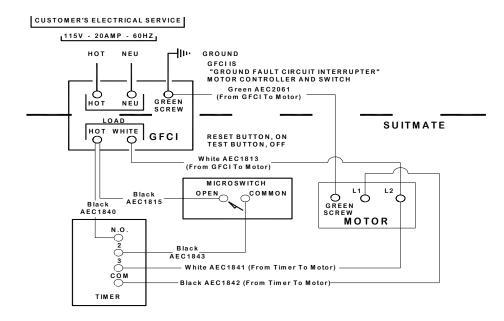
The SUITMATE<sup>®</sup>, equipped with a ground fault circuit interrupter (GFCI), which is designed to be connected to a 115 volt, 20 ampere 60 Hz *dedicated circuit* that is protected by a fuse or circuit breaker. *A PLUG-IN INSTALLATION IS NOT ACCEPTABLE!* The utilized circuit must be run to the SUITMATE<sup>®</sup> weatherproof Junction Box that contains the GFCI. A liquid tight raceway such as Ultralight<sup>®</sup> Liquid Tight Flexible Conduit (or the equivalent) should be used from
